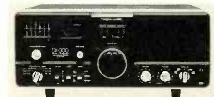
REALISTIC MODEL DX-300 communications receiver covers a frequency range between 10 kHz and 30 MHz.
