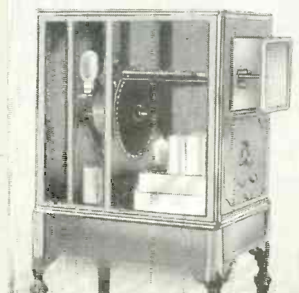
JENKINS PROJECTION RADIOVISOR, developed in 1931, used deForest's new neon-crater tube and a 1-inch scanning disc with sixty 1/2-inch lenses to throw a flying-spot image on the rear of the ground-glass viewing screen.
