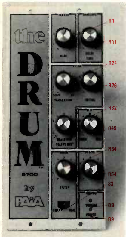
FIG. 9—THE FRONT PANEL of the 5700 synthesizer module with the codes keyed to the various controls.
