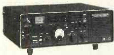
YAESU MODEL FRG-7000 covers a frequency range between 250 kHz to 29.9 MHz.
