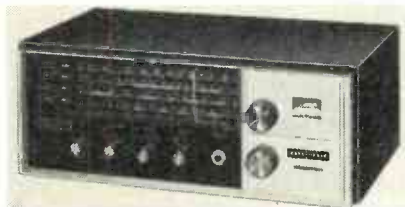
HEATH MODEL SW-717 4-band receiver covers 550 kHz to 30 MHz.
