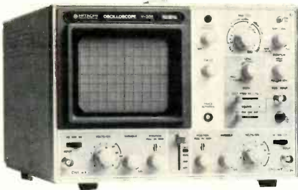
Hitachi Oscilloscope V-302 DC-30MHz dual-trace
